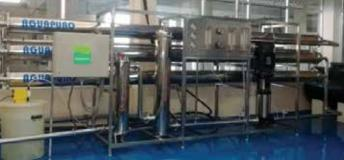
Aguapuro offers state of the art packaged Reverse Osmosis systems complete with pre & post treatment equipments offering very pure water form brackish or saline water.
